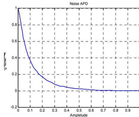
Fig.7 APD of noise due to Computer
