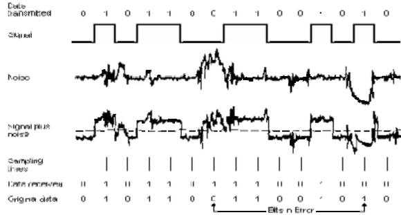
Fig.1. Effects of noise in digital communication.
