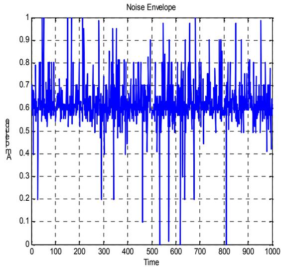
Fig. 4. Envelope of noise due to Mixer.
