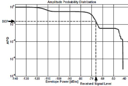
Fig. 3. The relation between APD and BER.
