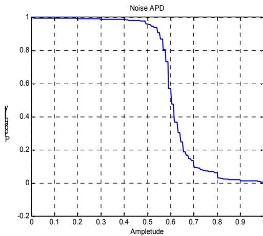
Fig. 5. APD of noise due to Mixer.
